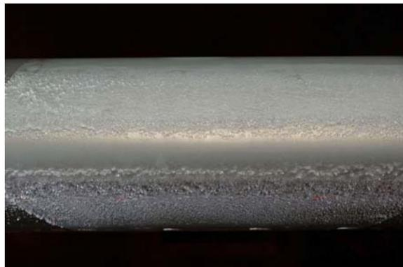
**Fig. 4** Tracing and photograph of roughness shape #1 EG1126. Tracing taken from ice casting used for aerodynamic testing with pressure orifice locations indicated by open circles.
