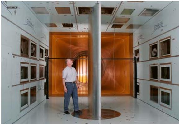
**Fig. 1 Photograph of NACA 23012 airfoil model installed in ONERA F1 wind-tunnel test section.**
