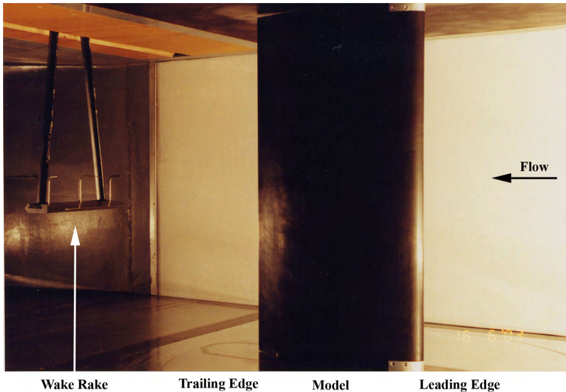
Figure 13. Experimental set-up for aerodynamic testing.
