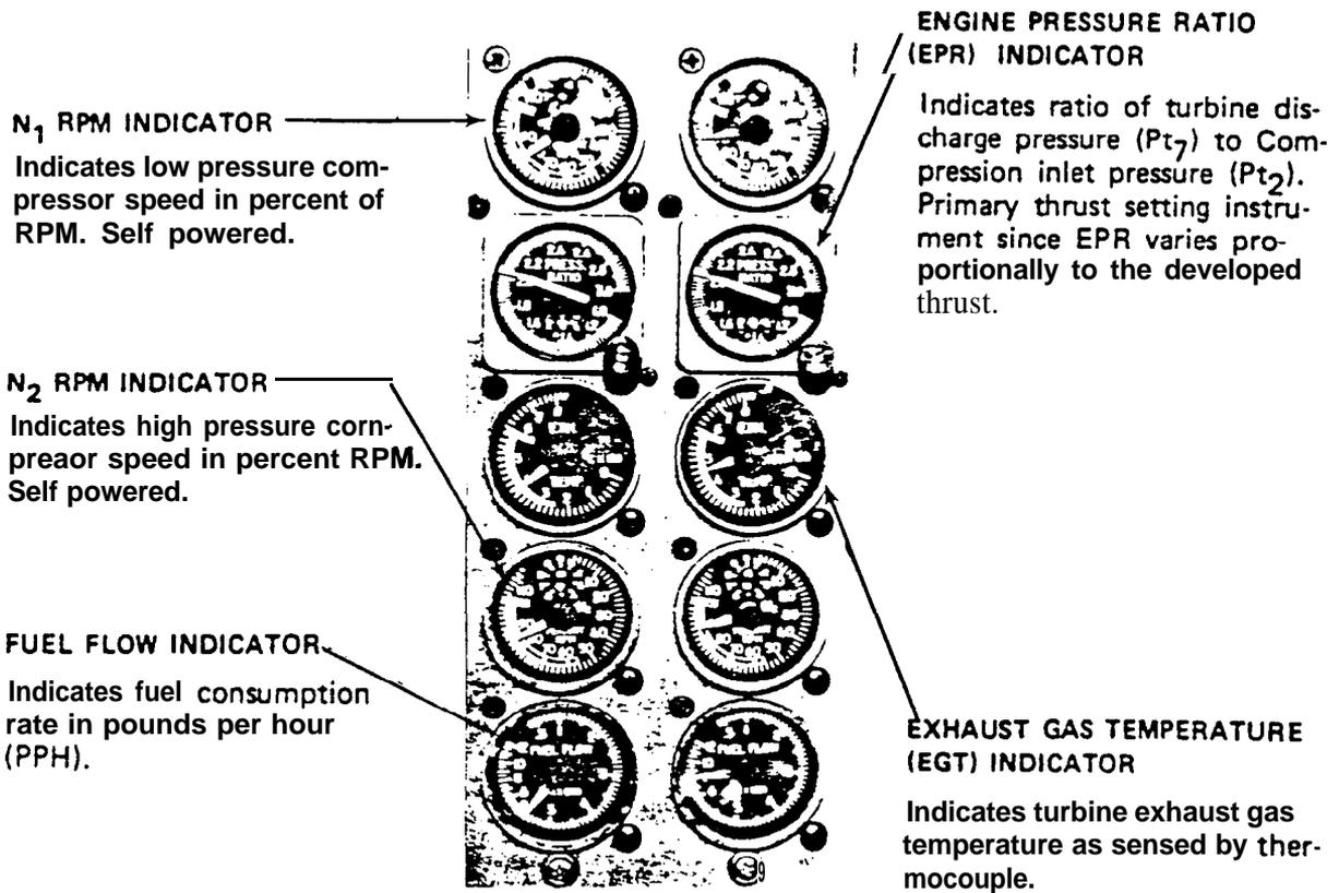
Figure 5. -- Center instrument panel functions.
