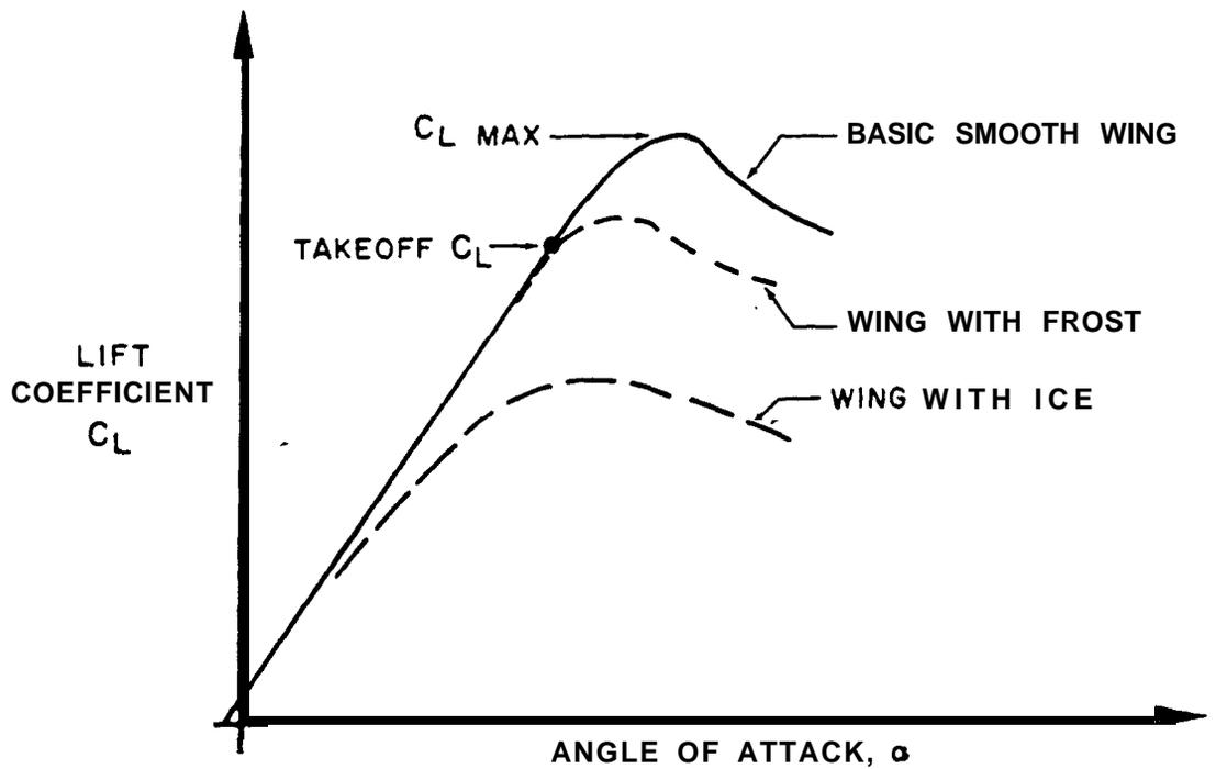
Where total lift developed by wing equals  $(L) = C_L \frac{1}{2} \rho V^2 S$
